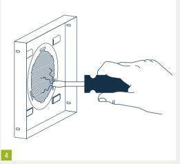
The filter insert is harmonized with Tecanno air vents and can be inserted into all recessed and surface-mounted vents (100/125).
