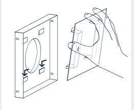
Hold the cover firmly on the right and left side. With your index and middle fingers, guide the vent cover tabs to the slots and insert them. Hold the cover at a slight angle.
